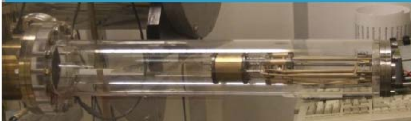
Simple ICR cell inside a vacuum tube
