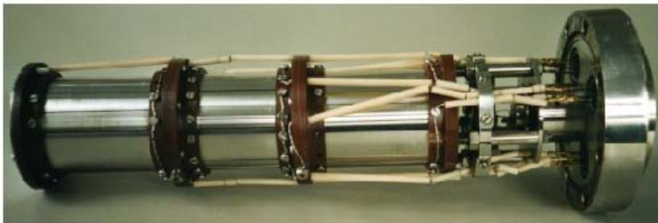
Multi section ICR cell with correction ring electrodes
